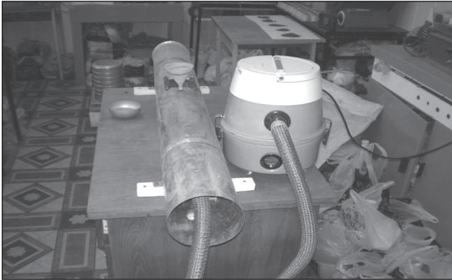
Laboratory aerodynamic unit for the study of wind erosion resistance of soil
