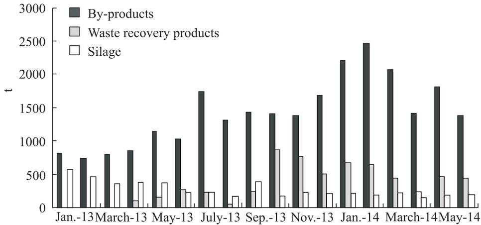
**Fig. 1.** The share of the main groups of substrates, used in the agricultural biogas station Kostkowice, at the Experimental Station of the National Research Institute of Animal Production in Grodziec Śląski
